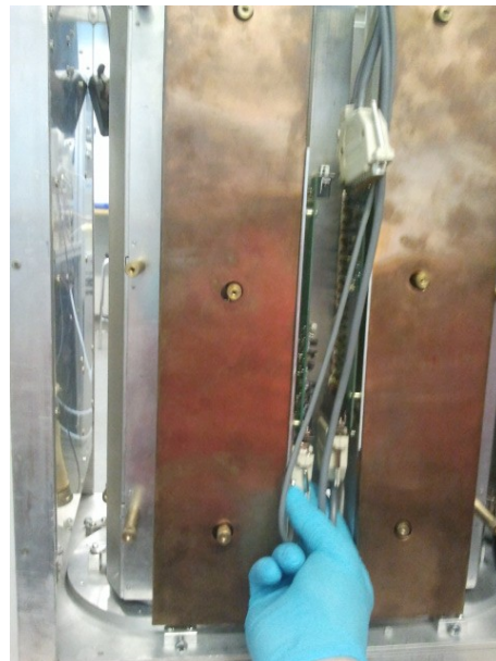
3 – connect back the electronic connectors.
